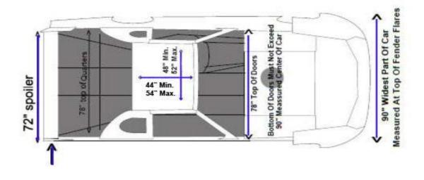
FRONT ROOF SUPPORTS 4" MAX. WITH 12" FLARE MAX. AT BOTTOM. REAR ROOF SUPPORTS OR "C" PILLARS WITH WINDOW OPENINGS ALLOWED BUT MUST BE SAME SIZE OPENING ON LEFT AND RIGHT SIDE, AND CANNOT BE OFFSET. CURVED OR ARCED ROOF SUPPORTS ALLOWED. 3" MAX. ARC ALLOWED AT WIDEST POINT, CHECKED WITH STRAIGHT EDGE EXTENDED FROM ROOF EDGE TO DOOR EDGE.
