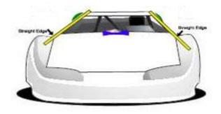
All body components 3" Min. above ground. All body measurements are maximum unless otherwise specified.
