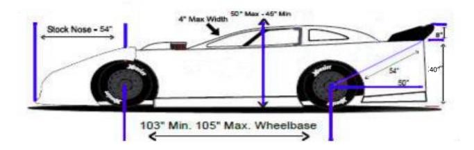
Rear deck height measured from ground to top of T-Bar is 40" with driver in car. The measurement of the spoiler is 8" from deck to top of spoiler.
