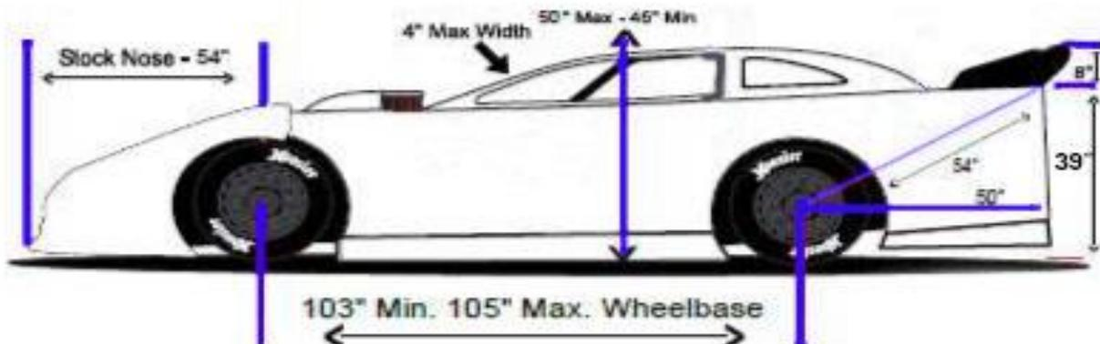
REAR DECK HEIGHT MEASURED FROM GROUND TO TOP OF T-BAR IS 39" MAXIMUM WITH DRIVER IN CAR. THE MEASUREMENT OF THE SPOILER IS A TOTAL OF ALL MATERIAL INCLUDING ANY TURNS UP OR DOWN AND INCLUDES SUPPORT BRACE
