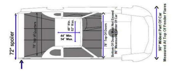
FRONT ROOF SUPPORTS 4" MAX. WITH 12" FLARE MAX. AT BOTTOM. REAR ROOF SUPPORTS OR "C" PILLARS WITH WINDOW OPENINGS ALLOWED BUT MUST BE SAME SIZE OPENING ON LEFT AND RIGHT SIDE, AND CANNOT BE OFFSET. CURVED OR ARCED ROOF SUPPORTS ALLOWED. 3" MAX. ARC ALLOWED AT WIDEST POINT, CHECKED WITH STRAIGHT EDGE EXTENDED FROM ROOF EDGE TO DOOR EDGE.
